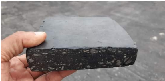
Samples for Hardness testing (100 mm X 100 mm X 25 mm)
